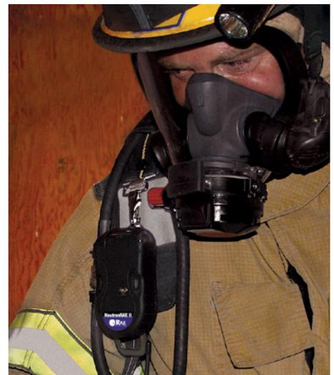
A First Responder uses the RAE Systems NeutronRAE II for audible and flashing alerts about the presence of a radiation threat and tracking of total dose exposure from gamma radiation.
